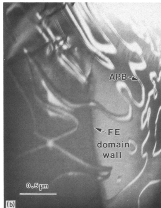
Figure 9 (a) BF micrograph illustrating ferroelectric domains in PST at -150^\circ\text{C} . (300 kV image obtained with EM7 microscope). (b) BF micrograph showing both ferroelectric domains and the APBs associated with structural order in PST at -150^\circ\text{C} . (300 kV image obtained with EM7 microscope).
